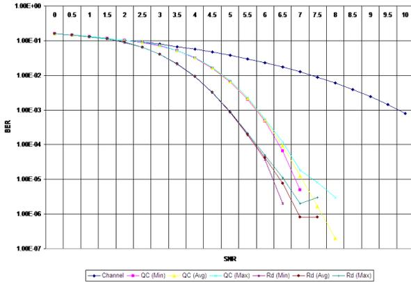
Fig. 3. Results for 1/2 LDPC rate using soft decoding
