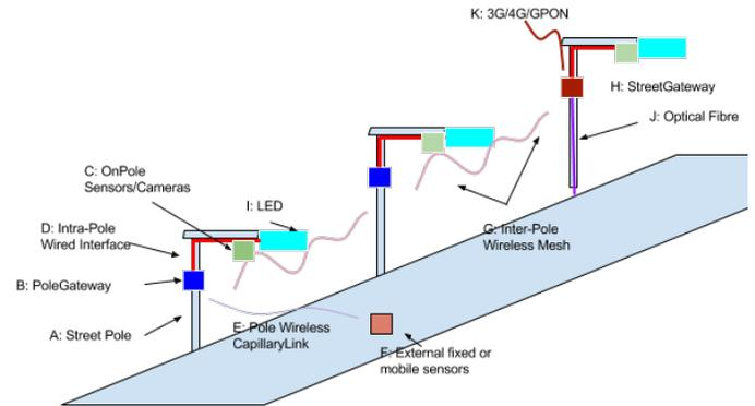
Figure 1: Streetlight Pole Test Bed Concept
