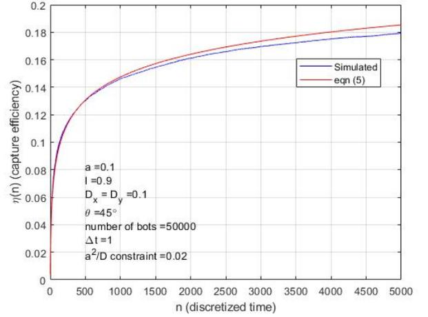
Fig. 3. Mathematical model and simulated capture efficiency
