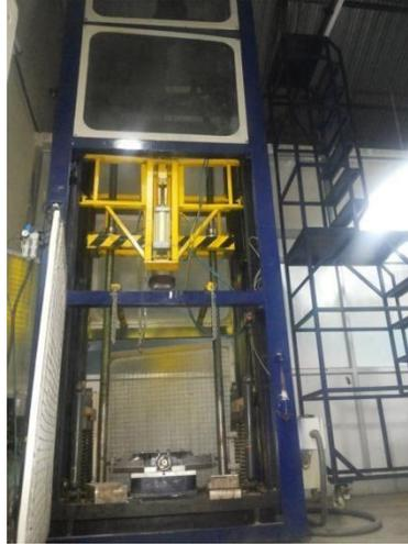
The initial slope of load-displacement is less in chamfer than square end because crushing starts at the chamfer part. Hoop ring shredded off and fail in tension (outer) and compression inner. Fragmentation and spaying mode are the two major failures. Hoop to axial ratio (H: A) is the amount of fiber in hoop direction and axial direction (more axial fiber more peak load for axial load) [8]. The main factors which affect the crush behavior are fiber, matrix, crushing speed and temperature.
