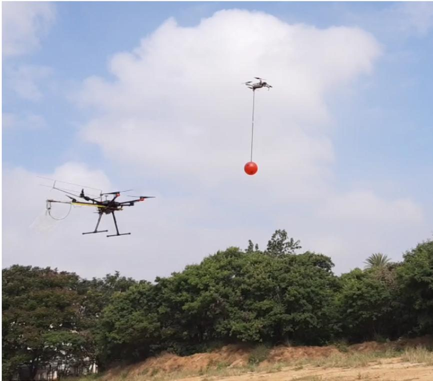
Fig. 1: Own UAV and target UAV. Using visual information, own UAV estimates and predicts the location of target
